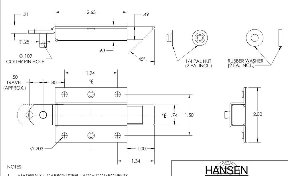
MATERIALS: CARBON STEEL LATCH COMPONENTS
